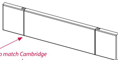
*V grooves on front to match Cambridge door design (no V grooves shown on reverse for other door ranges)*
