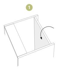
18mm back panel for added rigidity on base units, means you don't need to worry about your cookware damaging the backs!
