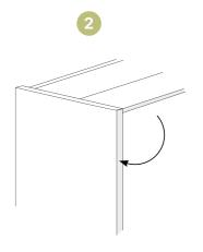
2mm PVC on leading edges prevents moisture from getting into the cabinet structure and causing damage.
